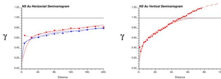
Figure 3 Normal scores variogram for gold in the plane of vein directions (left) and parallel to vein thickness (right). Blue line on the left corresponds to the dip direction, red line corresponds to the along-strike direction.
