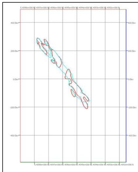
Figure 7 Section at 425405 Easting, looking east, comparing the 0.5 gpt gold grade shell from RBF (red) with the MG domain shell for an iso-probability of 40% (cyan).
