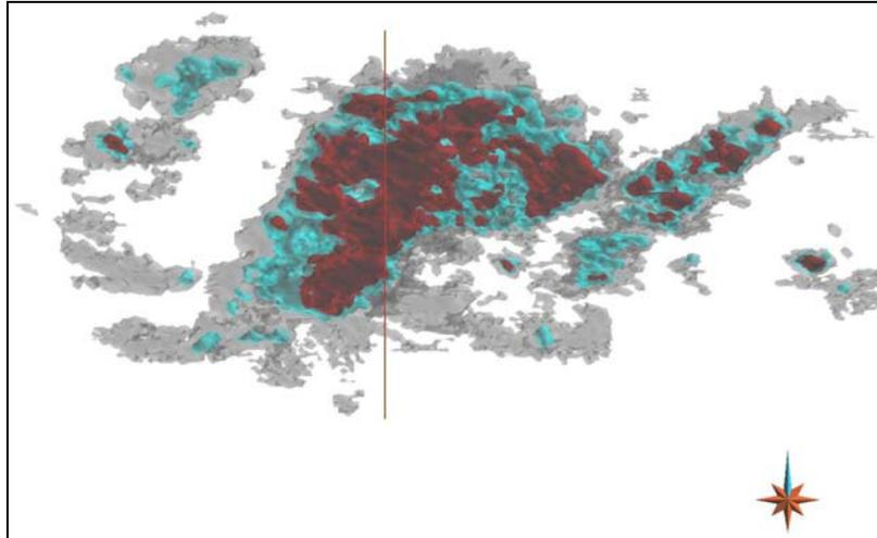
Figure 4 Comparison of iso-probability shells for 0.50 gpt grade shell: probability to exceed grade 0.5 gpt of 30% or higher (grey), 40% or higher (cyan), and 50% or higher (red). Red vertical line corresponds to location of 2D section shown in Figure 5.
