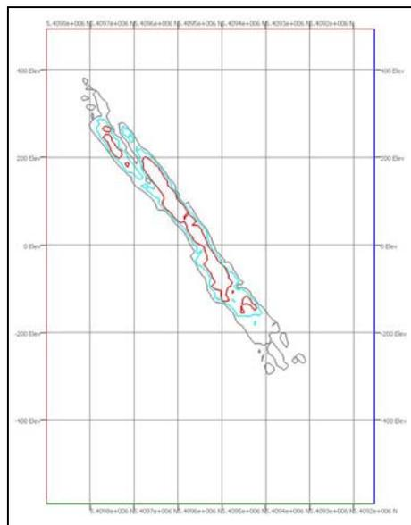
Figure 5 Section at 425405 Easting, looking east, illustrating the nesting of iso-probability shells for 0.50 gpt grade threshold: probability to exceed grade 0.5 gpt of 30% or higher (grey), 40% or higher (cyan), and 50% or higher (red).
