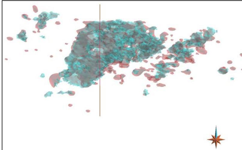
Figure 6 Comparison of 0.50 gpt gold grade shell from RBF (red) and a similar shell using MG domaining for an iso-probability of 40% (cyan). Red vertical line corresponds to location of 2D section shown in Figure 7.
