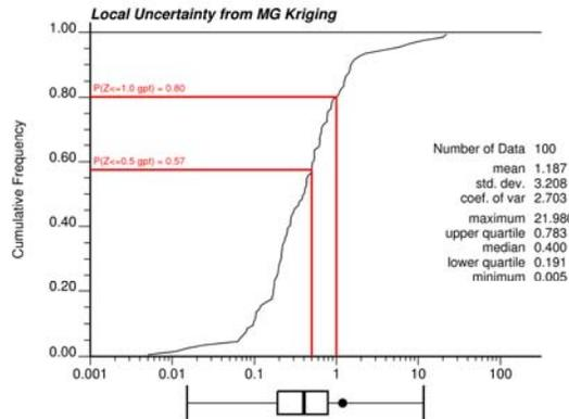
Figure 1 Determination of probability to exceed a grade threshold using the local distribution of grade uncertainty accessible via MG kriging.
